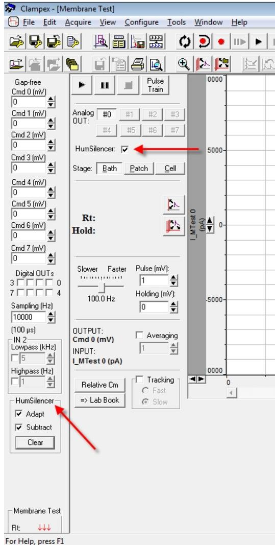
**Figure 4-6: HumSilencer system controls in the Real Time Controls panel and Membrane Test dialog**
