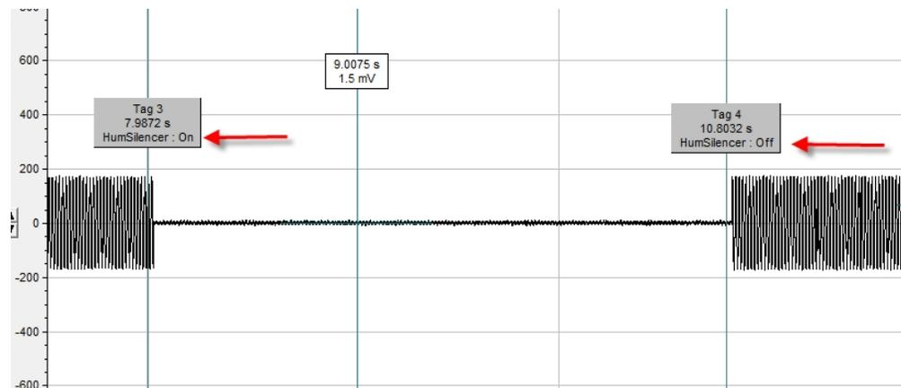
**Figure 4-4:** HumSilencer Start and HumSilencer Stop comment tags displayed in an open data file.
