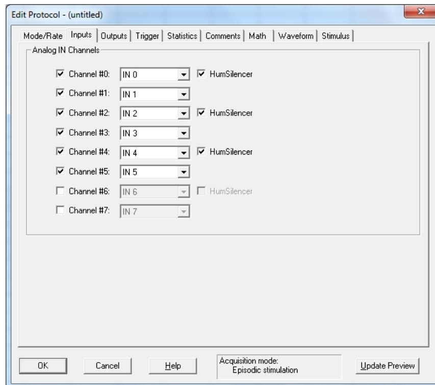
**Figure 4-1: Edit Protocol > Input dialog tab check box used to enable the Real Time Controls for the HumSilencer system**
