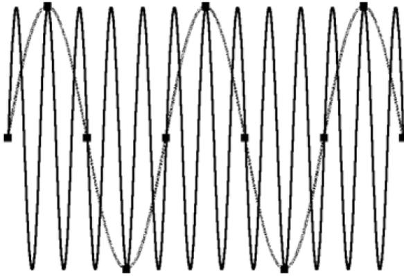
**Figure 2-2: Illustration of aliasing.**
