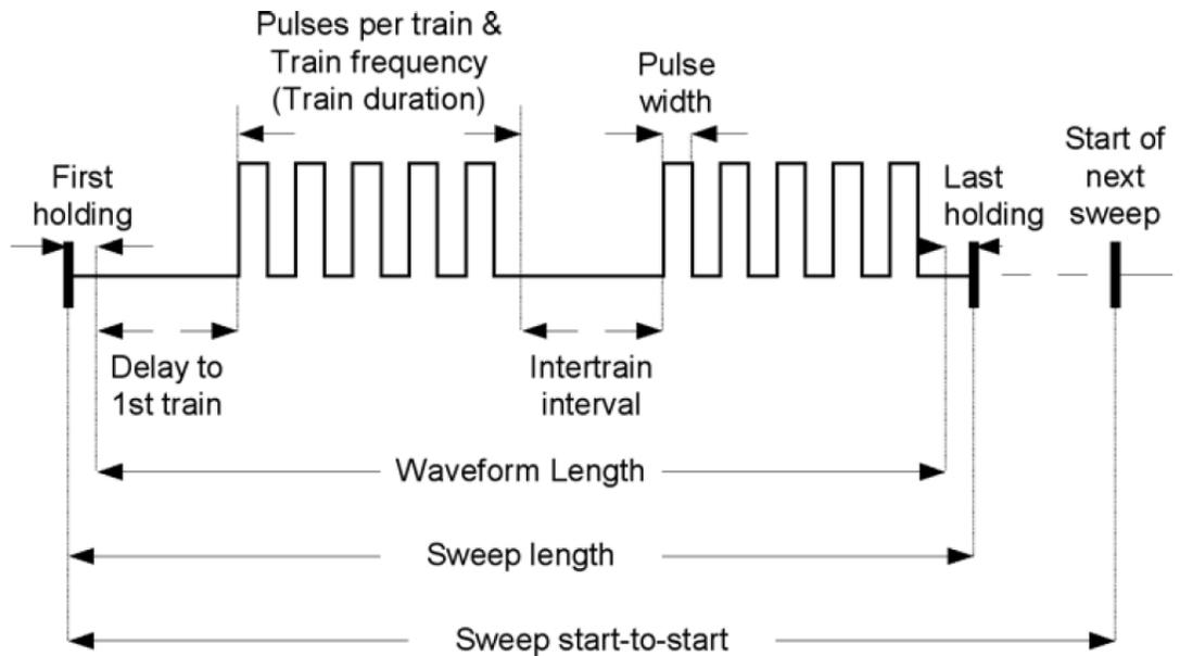
**Figure 4-10: Conditioning sweep configuration with two trains per sweep, showing parameters used on Conditioning tab.**
