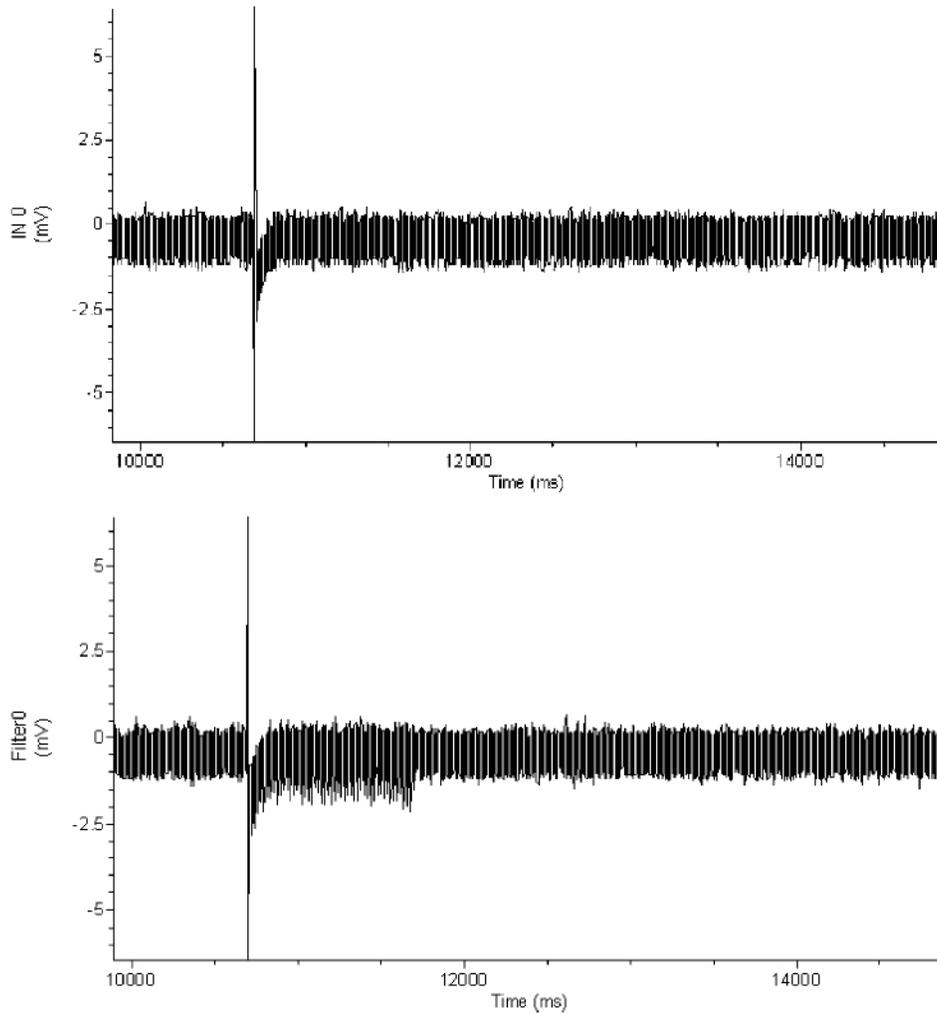
**Figure 8-24: EI filtering showing introduction of false line harmonics.**
