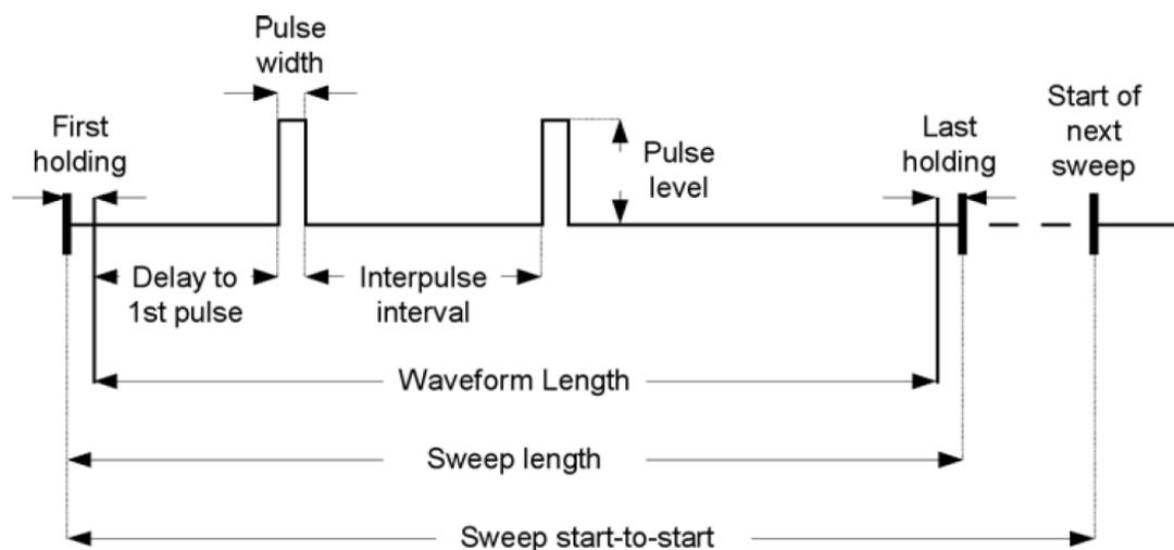
**Figure 4-9: Baseline sweep with two pulses per sweep showing configuration parameters used on Baseline tab.**
