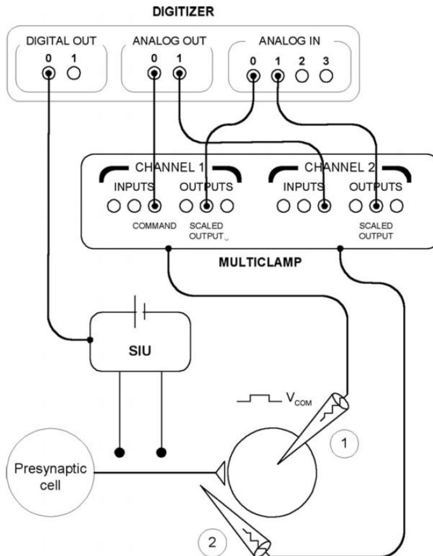
**Figure 4-8: Example of LTP experiment setup, with digital presynaptic stimulation, postsynaptic intracellular voltage step command and current recording, and extracellular recording.**
