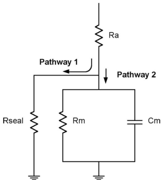
**Figure 4-7: Idealized circuit showing two pathways from electrode tip to ground.**
