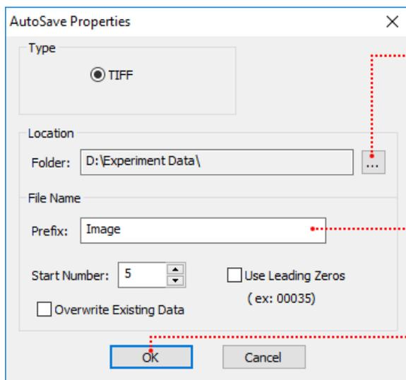
The screenshot shows the "AutoSave Properties" dialog box. It has a "Type" section with "TIFF" selected. The "Location" section shows a "Folder" field with "D:\Experiment Data\" and an ellipsis icon. The "File Name" section shows a "Prefix" field with "Image". Below this are "Start Number" (5) and "Use Leading Zeros" (unchecked) with an example "(ex: 00035)". There is also an "Overwrite Existing Data" checkbox. At the bottom are "OK" and "Cancel" buttons.
